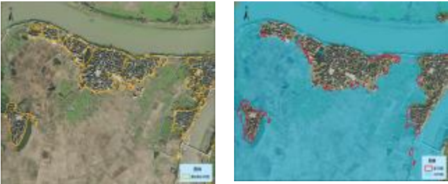
图3 沿河房屋受淹范围提取分析(鄱阳县昌洲乡南林村) Fig.3 Extraction and analysis of inundated buildings along Poyang Lake
