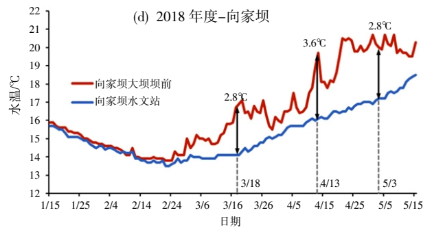
图11 2017、2018年溪洛渡、向家坝坝前及坝下水温变化过程对比 Fig.11 The variation comparison of water temperature in front of and below Xiluodu and Xiangjiaba dam in 2017 and 2018
