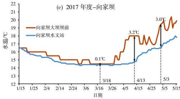
图11 2017、2018年溪洛渡、向家坝坝前及坝下水温变化过程对比 Fig.11 The variation comparison of water temperature in front of and below Xiluodu and Xiangjiaba dam in 2017 and 2018
