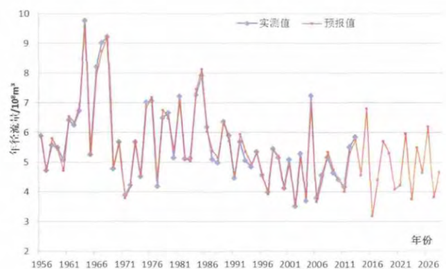
图4 白云站实测流量与拟合(预测)流量过程线对照图 Fig.4 The comparison between the observed runoff and fit (predictive) runoff at the Baiyun station
