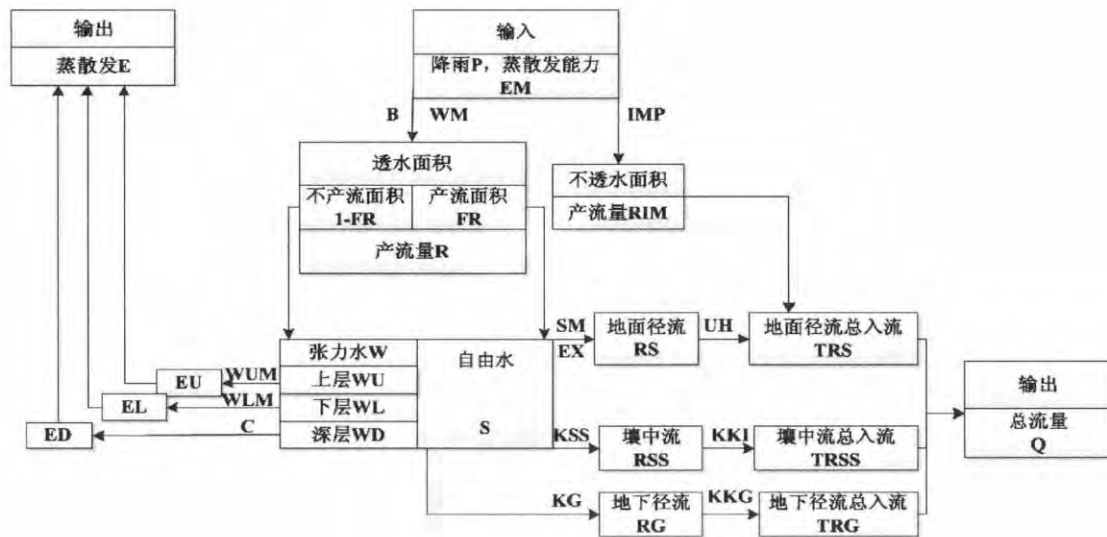
图2 三水源新安江模型结构图 [12] Fig.2 The structure of the Xin'anjiang model
