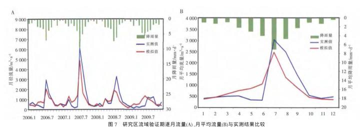
Fig.7 Comparison between the observed and simulated results of the monthly rainfall-runoff simulation(A) and monthly mean runoff simulation(B) for the Huaihe River basin during the validation period
