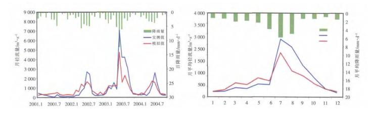
图 5 研究区流域率定期逐月流量(A)、月平均流量(B)与实测结果比较 Fig.5 Comparison between the observed and simulated results of the monthly rainfall-runoff simulation(A) and monthly mean runoff simulation(B) for the Huaihe River basin during the calibration period
