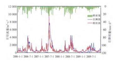
图 6 淮河流域验证期(2006~2009 年)日降雨、径流模拟与实测结果比较 Fig.6 Comparison between the observed and simulated results of the daily rainfall-runoff simulation for the Huaihe River basin during the validation period (2006~2009)
