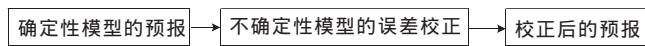
图1 提高短期水文预报精度的耦合方式 Fig.1 The coupling way of deterministic and nondeterministic method for the accuracy of short time forecast
