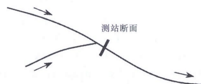
图 3 水位流量关系受支流来水影响 Fig.3 Stage discharge relation effected by tributary inflow
